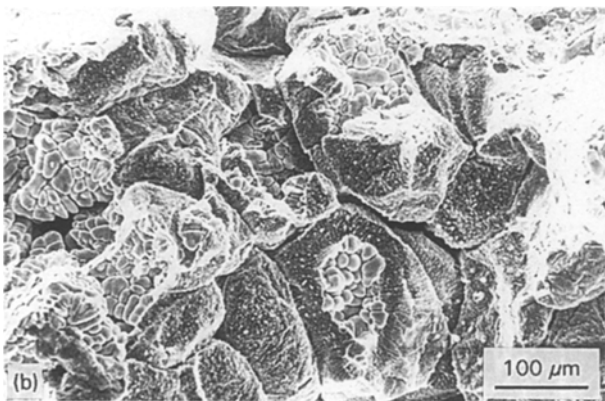
Figure 8 Scanning electron micrographs showing the fracture surface tested at 300 °C and 0.02 s -1 ; (a) intergranular fracture; (b) interdendritic and intergranular fracture.
